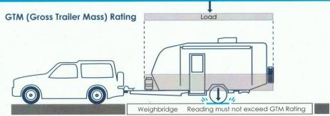
GTM (Gross Trailer Mass) Rating - The total permissible mass that can be supported by the wheels/ tyres of the Caravan. This includes whatever you add as payload (e.g. water, gas, equipment and luggage), but does not include the mass supported by the tow vehicle. The GTM Rating must not be exceeded.
