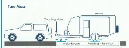
Tare Mass - The total weight of the Caravan (load on tyres plus coupling load) with all options and fittings as supplied by the manufacturer, with empty water tanks, gas bottles, excluding fluids not essential for operation on public roads, and without luggage or personal effects.
