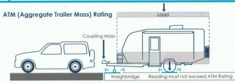
ATM (Aggregate Trailer Mass) Rating - The total permissible mass of the Caravan. This includes the coupling mass and whatever you add as payload (e.g. water, gas, luggage) up to the specified rating. The ATM Rating must not be exceeded.
